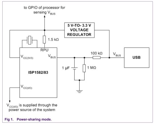
In power-sharing mode, the processor will experience continuous interrupt when  $V_{BUS}$  is lost; see <u>Fig 2</u>. This is because the default status of the interrupt pin when operating in sharing mode with  $V_{BUS}$  not present is LOW. To overcome this, implement external  $V_{BUS}$  sensing circuitry. The output from the voltage regulator can be connected to pin GPIO of the processor to qualify the interrupt from the ISP1582/3.
